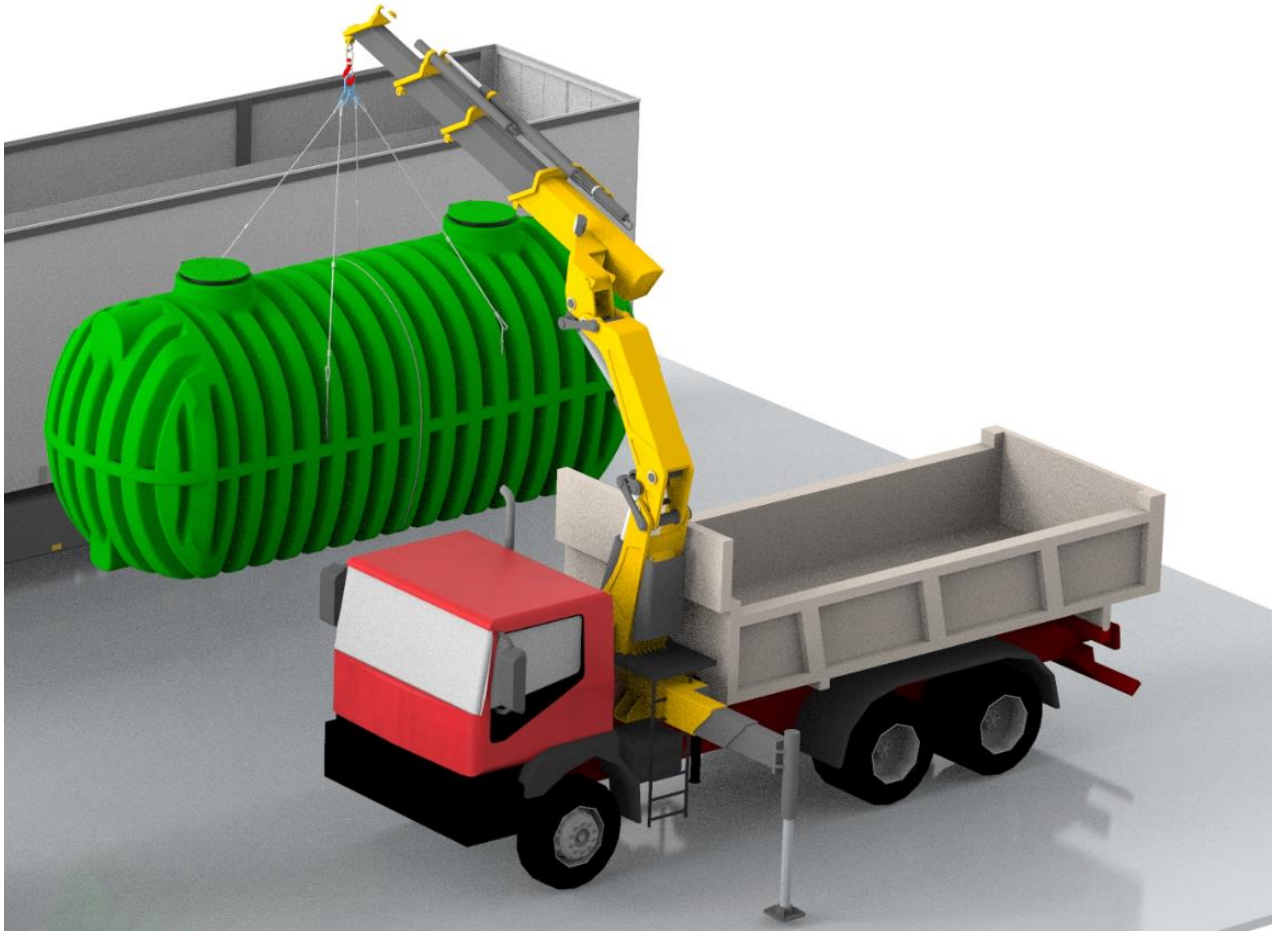
Picture 2 (Lifting the tank with 4 Slings and excavator.
